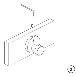
**3** Place assembly over the mounting bracket with set screws facing down. Tighten the set screws.
