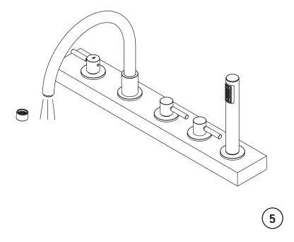
After installing faucet, remove aerator and open the hot and cold supplies. Check for leaks. Turn on faucet handle for one minute to flush debris from faucet. Turn off the water supply, install the canopy and handle, then reassemble the aerator.
