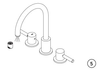
5 Remove aerator and turn on water to remove any left over debris. Re-assemble aerator.
