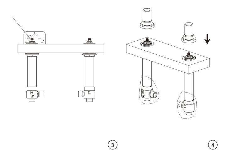
Adjust position of the bodies relying on specific gauge (A, B, D) supplied as the figure indicated to make sure they can fit with the trim in various ranges. After that, tighten fixing nuts from below by wrench.
