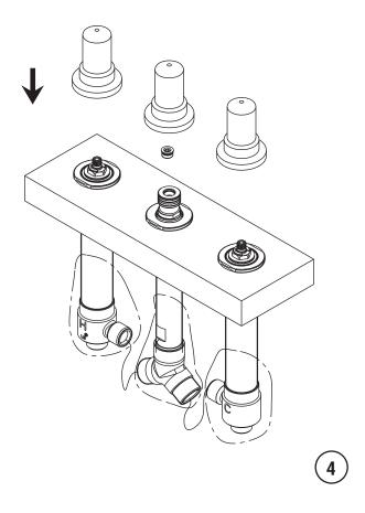
4 Replace the protective bubble bag and cap to body assembly to prevent dirt entering during job constructing, and replace plug to spout tube assembly to prevent leakage during job constructing.
