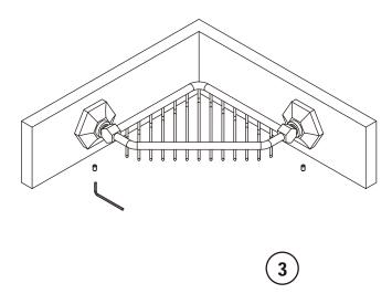
3 Place assembly over the mounting bracket with set screws facing down. Tighten the set screws.
