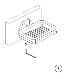
**3** Place assembly over the mounting bracket with set screws facing up. Tighten the set screws.
