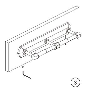
3 Place assembly over the mounting bracket with set screws facing up. Tighten the set screws.
