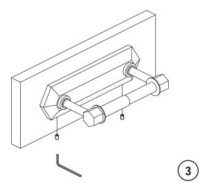
3 Place assembly over the mounting bracket with set screws facing up. Tighten the set screws.
