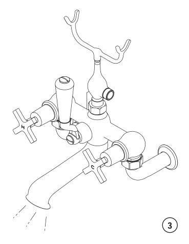
**3** After installing faucet, open the hot and cold supplies to check for leaks. Turn on faucet handle for one minute to flush debris from faucet. Turn off the handle.
