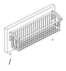
3 Place assembly over the mounting bracket with set screws facing down. Tighten the set screws.
