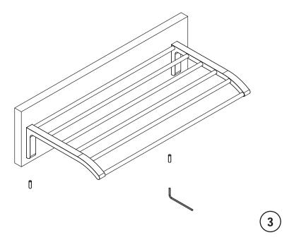
3 Place assembly over the mounting bracket with set screws facing down. Tighten the set screws.
