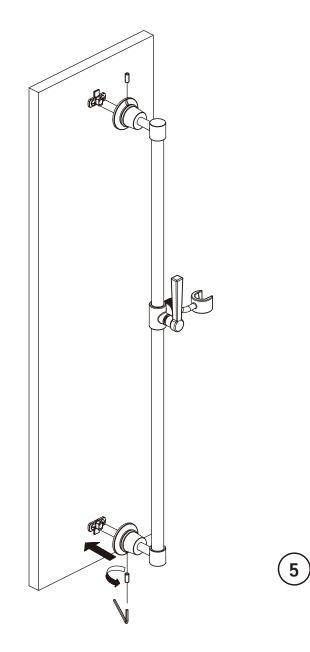
**5** Place assembly over the mounting bracket. Tighten the set screws.
