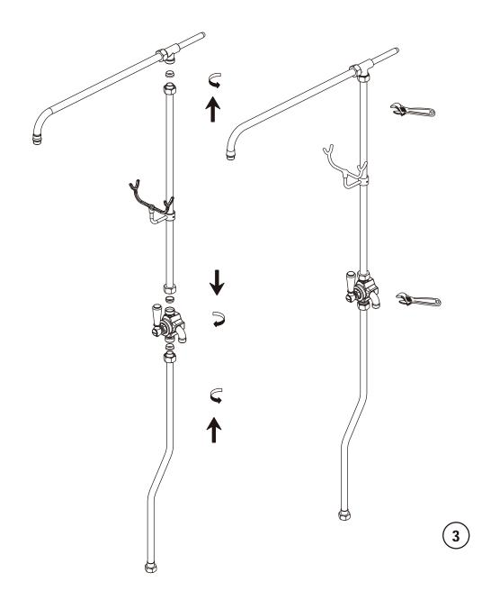
**3** Put the compression olive into the riser bracket and then fix the riser with the bracket. Put the compression olive into the diverter body and then fix the riser with the diverter body. Tighten the nut by wrench in order to fix the riser with the bracket and with the diverter body.
