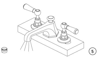
**5** After installing faucet, open the hot and cold supplies to check for leaks. Turn on faucet handle for one minute to flush debris from faucet. Turn off the handle.
