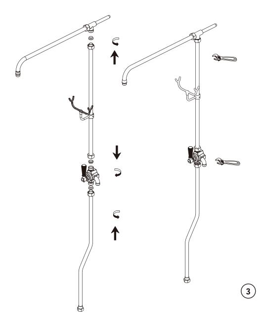
Put the compression olive into the riser bracket and then fix the riser with the bracket. Put the compression olive into the diverter body and then fix the riser with the diverter body. Tighten the nut by wrench in order to fix the riser with the bracket and with the diverter body.
