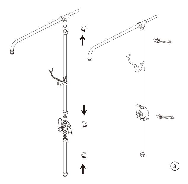
Put the compression olive into the riser bracket and then fix the riser with the bracket. Put the compression olive into the diverter body and then fix the riser with the diverter body. Tighten the nut by wrench in order to fix the riser with the bracket and with the diverter body.
