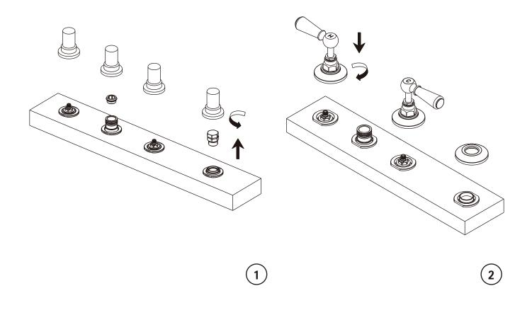
1 Make sure that main water supply is shut off before further installation. Take off all rubber protective caps, plugs from valves, as well as the underneath protective bubble bags.
