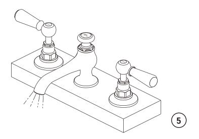
**5** After installing faucet, open the hot and cold supplies to check for leaks. Turn on faucet handle for one minute to flush debris from faucet. Turn off the handle.
