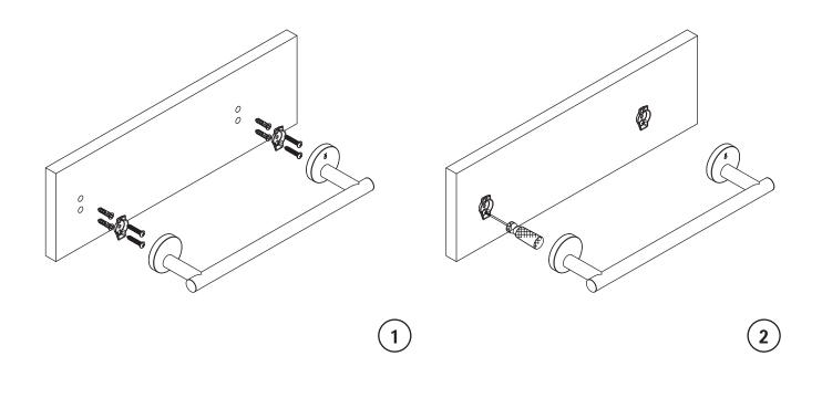
Position the mounting bracket on the wall where required. Please note the direction of the mounting bracket should be as shown. Mark the location of mounting screws. Drill holes in the wall to fit the anchors. Tap the plastic anchor into the hole with a hammer. 2 Position the mounting bracket to be mounted on the wall, then thread the fixing screws through the mounting hole into the plastic anchor. Turn the screws slowly until they are tight.
