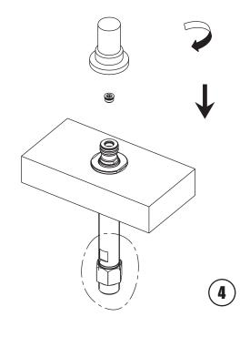
Adjust position of the body relying on specific gauge (A, B, C) supplied as the figure indicated to make sure it can fit with the trim in various ranges. After that, tighten fixing nuts from below by wrench. Gauge A (027105) for M2-1029. Gauge B (027104) for K1-1030. Gauge C (027107) for M1-1029.
