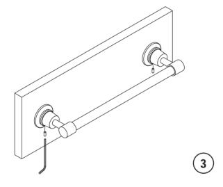
Place assembly over the mounting bracket with set screws facing down. Tighten the set screws.
