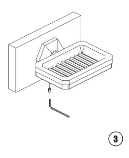
Place assembly over the mounting bracket with set screws facing up. Tighten the set screws.
