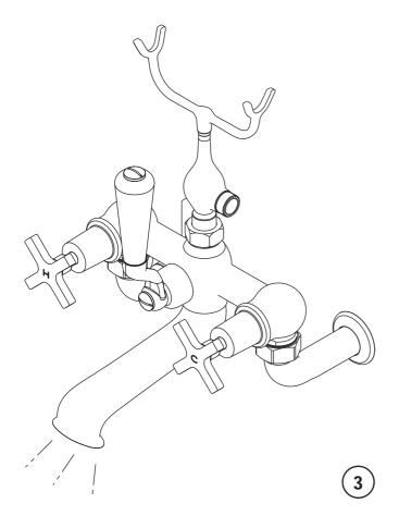
**3** After installing faucet, open the hot and cold supplies to check for leaks. Turn on faucet handle for one minute to flush debris from faucet. Turn off the handle.
