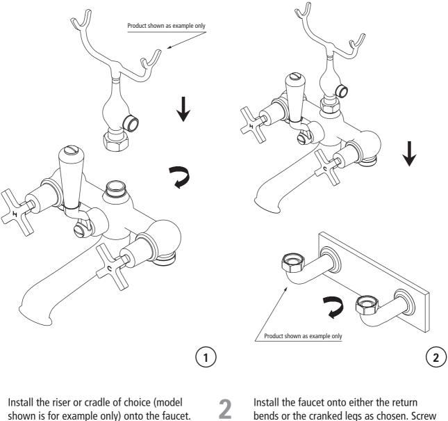
Screw the nut tightly to seal securely.
