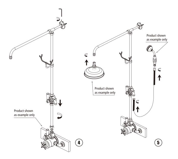
Fix riser kit to the faucet of choice (model shown is for example only). Then fix the riser kit with the Wall bracket by fixing the set screw. Finally fix the wall bracket to wall where is appropriate by anchors and screws. **5** Connect the shower head of choice (model shown is for example only) with shower arm. Connect the flexible hose with hand shower of choice (model shown is for example only) with diverter body.
