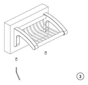
Place assembly over the mounting bracket with set screws facing down. Tighten the set screws.
