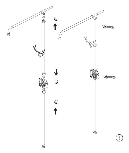
Put the compression olive into the riser bracket and then fix the riser with the bracket. Put the compression olive into the diverter body and then fix the riser with the diverter body. Tighten the nut by wrench in order to fix the riser with the bracket and with the diverter body.
