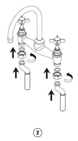
Take out product from the box. Turn the spout to the right front position as the figure instructed. Tighten the fixing set screw to secure the spout fixed. Install the faucet onto either the return bends or the cranked legs as chosen. Attach the legs to the faucet but do not screw the nut up tightly yet.
