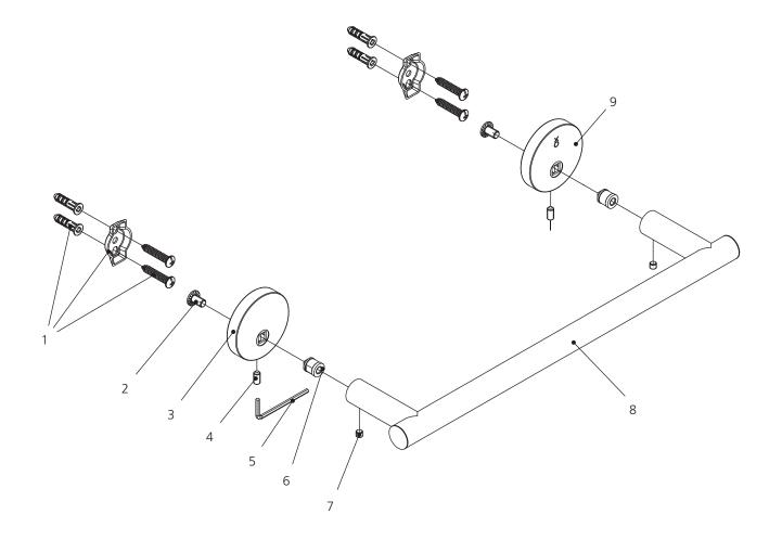
1Fixing kit (290033)2Screw (008711)3Wall plate (L) (240303H)4Set screw (053009)5Allen key (031000)6Adaptor (259120)7Screw (008005)8Rail assembly (250375)9Wall plate (R) (240303C)
