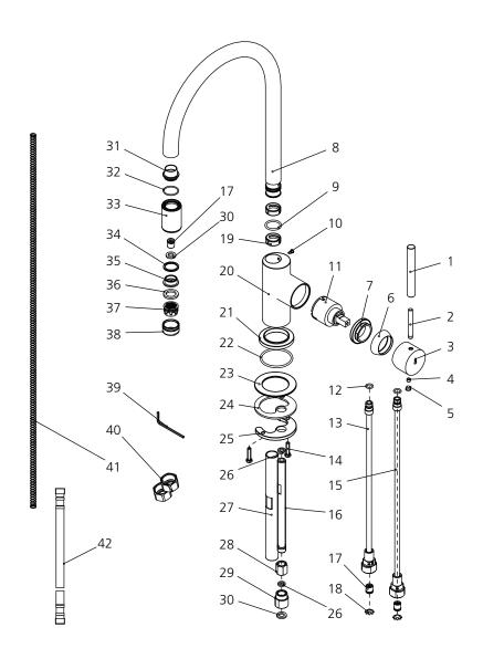
1 Handle sleeve (038105) 2 Handle Stem (108926) 3 Handle base (215494) 4 Screw (292505) 5 Plug (028079) 6 Cap (103319) 7 Adjusting ring (104233) 8 Spout (139636) 9 O-ring (004010N) 10 Screw (085526) cartridge (507348N) 11 O-ring (004001N) 12 Copper pipe assembly (064239W) 13
