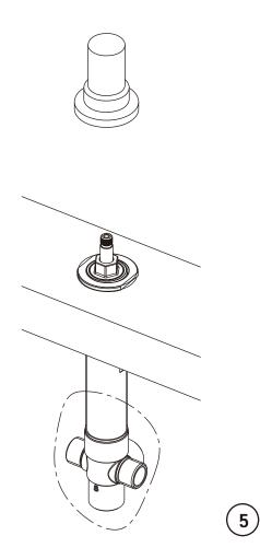
**5** Replace the protective bubble bag and protective caps to prevent dirt ingress or water leakage during construction.
