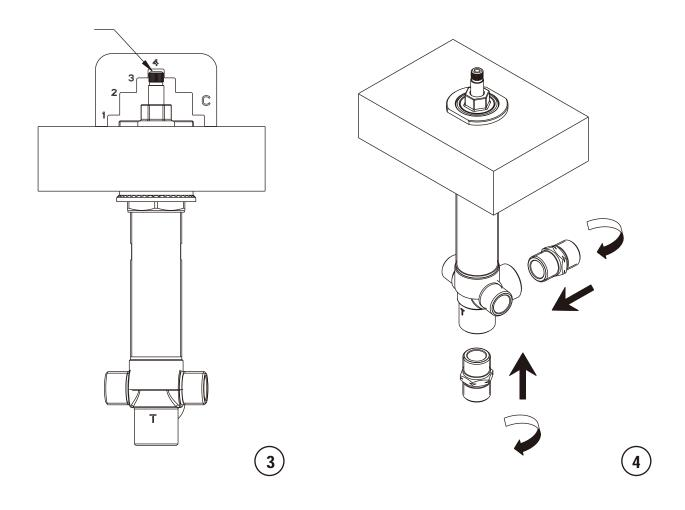
**3** Adjust position of the bodies relying on specific gauge (B, C) supplied as the figure indicated to make sure they can fit with the trim in various ranges. After that, tighten fixing nuts from below by wrench.
