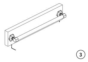
3 Place assembly over the mounting bracket with set screws facing down. Tighten the set screws.
