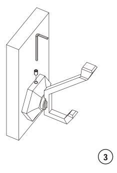
3 Place assembly over the mounting bracket with set screws facing up. Tighten the set screws.
