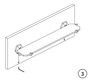
3 Place assembly over the mounting bracket with set screws facing down. Tighten the set screws.
