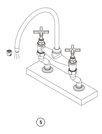
After installing faucet, remove aerator and open the hot and cold supplies.
