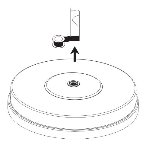
Wrap Teflon tape around the threads of the connecting pipe in a clockwise direction. Thread the shower head on the tape of the pipe and hand tighten as tight as possible.
