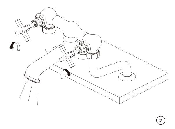
2 After installing faucet, open the hot and cold supplies to check for leaks. Turn on faucet handle for one minutes to flush debris from faucet. Turn off the handle.
