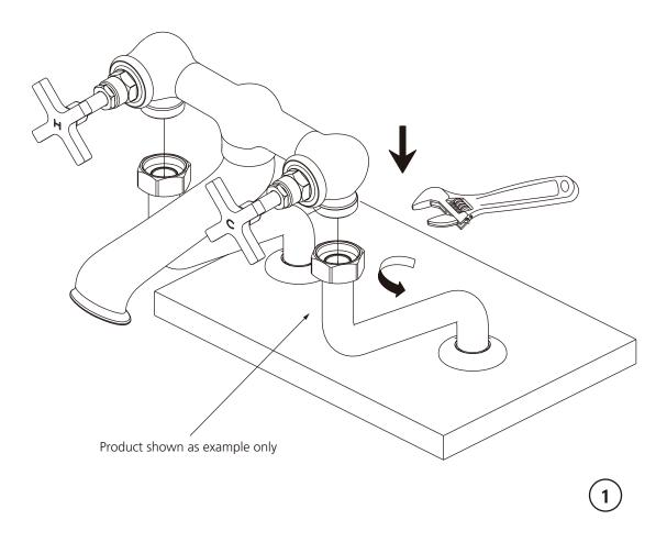
1 Install the faucet onto either the return bends or the cranked legs as chosen. Screw the nut tightly to seal securely.
