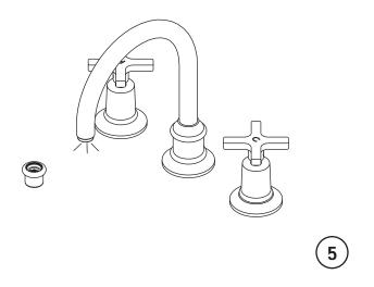
5 Remove aerator and turn on water to remove any left over debris. Re-assemble aerator.
