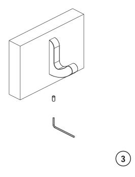
3 Place assembly over the mounting bracket with set screws facing down. Tighten the set screws.
