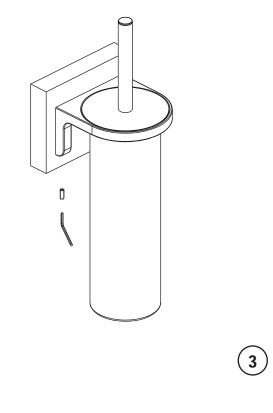
**3** Place assembly over the mounting bracket with set screws facing down. Tighten the set screws.
