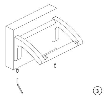
3 Place assembly over the mounting bracket with set screws facing down. Tighten the set screws.
