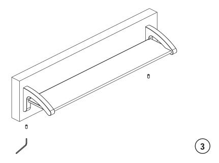
3 Place assembly over the mounting bracket with set screws facing down. Tighten the set screws.
