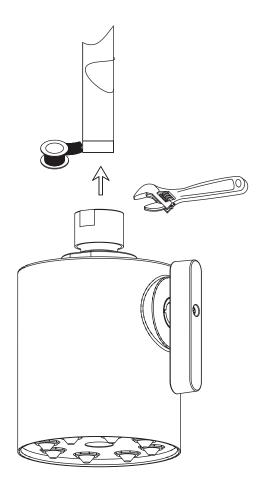
Apply pipe tape on the threads of shower arm (which is not included in this product package). Tighten the shower head to shower arm with wrench.
