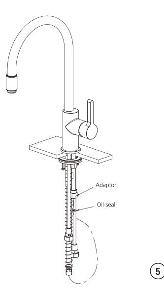
5 Attach oil-seal to the adaptor. Then connect hose to the adaptor tightly.
