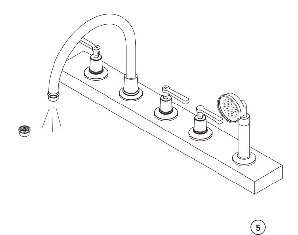
5 After installing faucet, remove aerator and open the hot and cold supplies. Check for leaks. Turn on faucet handle for one minute to flush debris from faucet. Turn off the water supply, install the canopy and handle, then reassemble the aerator.
