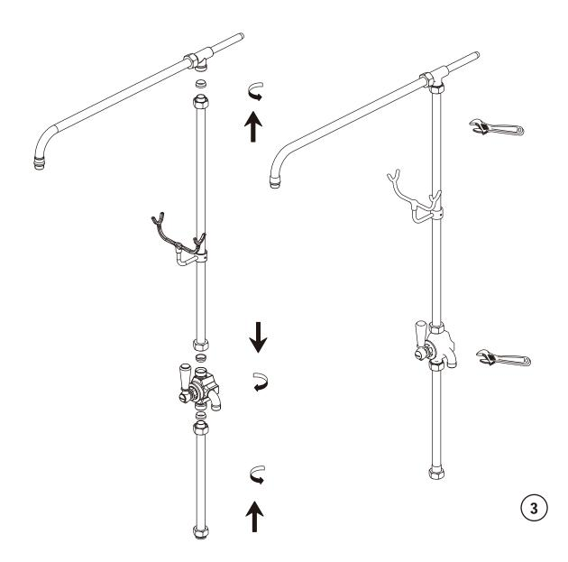
**3** Put the compression olive into the riser bracket and then fix the riser with the bracket. Put the compression olive into the diverter body and then fix the riser with the diverter body. Tighten the nut by wrench in order to fix the riser with the bracket and with the diverter body.
