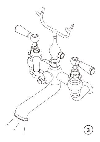
After installing faucet, open the hot and cold supplies to check for leaks.
