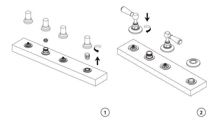
1 Make sure that main water supply is shut off before further installation. Take off all rubber protective caps, plugs from valves, as well as the underneath protective bubble bags.
