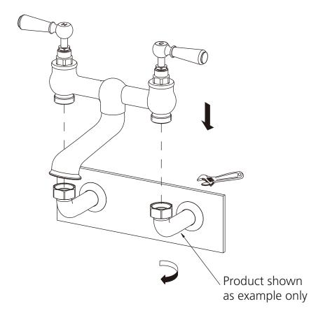
1 Install the faucet onto either the return bends or the cranked legs as chosen. Screw the nut tightly to seal securely.
