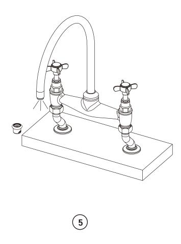
After installing faucet, remove aerator and open the hot and cold supplies.
